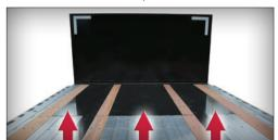
Steel counterweights are built into the front floor to balance the forklift weight when returning empty. For optimum performance make sure the counterbalance and 5th wheel spec are correct for your application.
