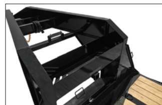
TOOL TRAY W/ WINCH RECEIVER MOUNT
