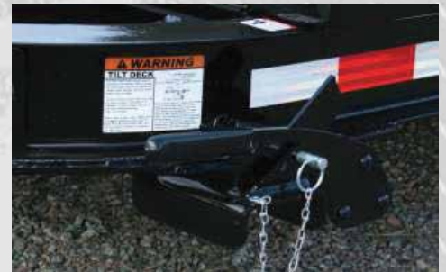
Single deck latch lever with dual latch securement is easy to operate.
